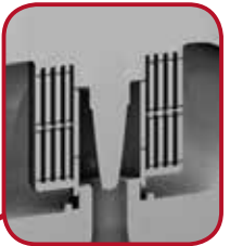
Valve stem and 5-stages control/throttle element 阀杆和五级控制节流元件
